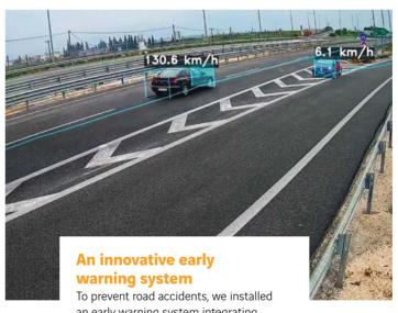
an early warning system integrating a camera and intelligent pattern recognition software on the Via Pribina expressway in Slovakia to detect vehicles entering the fast lane in the wrong direction and alert the driver. Since its launch, the system has achieved an 88% success rate, and plans are in place to extend it to other sections of the expressway.
